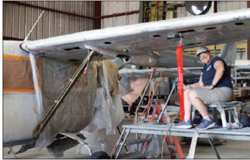
Cindy Ramsey polishing the wing on our C337 Skymaster
