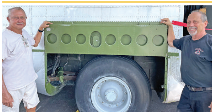
Larry Dickinson and Larry Knoch along with Bob Fillipi (not pictured) are restoring the C-123. They are proudly showing the corroded landing gear door that they remanufactured right down to the correct number of rivets. This is an example of the quality work the restoration team turns out: "Everything is in the details".
