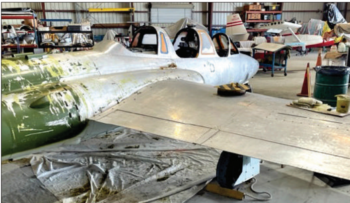
Stripping the paint to bare metal in progress
