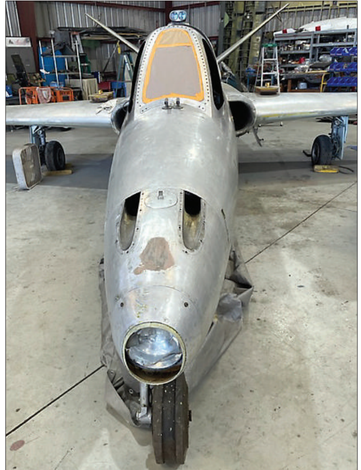
Stripping the bottom in progress, the two openings on the nose are for the mounting of 7.62 mm guns, yes we do have the mock-up guns on hand.
