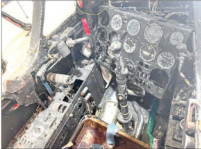
Cockpit to be removed, cleaned, painted and then reinstalled.
