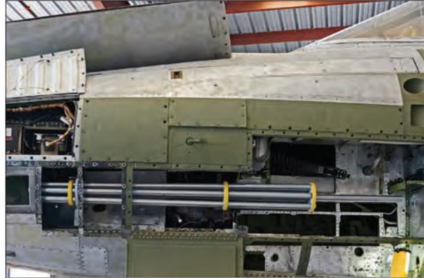
Restoration has started on the F-105. The nose mounted guns are being made from scratch...great job.
