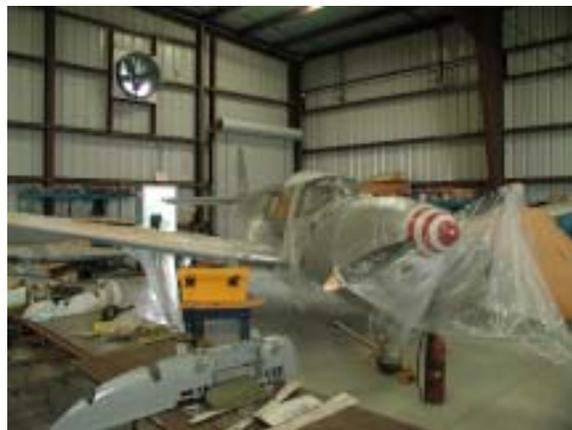
Messerschmitt 208 undergoing reassembly and paint
