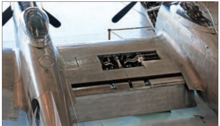
Ammo compartment for the XP-82's 6 machine guns. Each of the .50 cal machine guns carried 400 rounds.
