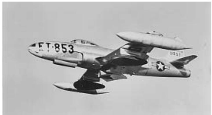
NAPALM CARRIER...One hundred and fifty gallons of flaming death, seventy-five gallons of napalm in each of the dark colored wing tanks, speeds on its way toward enemy lines in Korea through courtesy of an F-80 jet fighter of the U.S. Far East Air Forces. National Archives Photo
